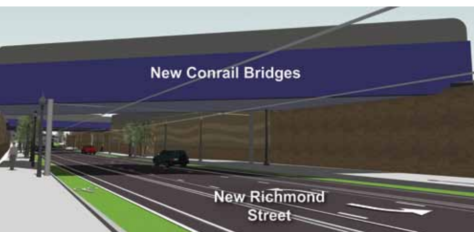
GR1 improvements include the low-hanging Conrail construction of four smaller bridges to replace overpasses on Richmond Street near Lehigh Avenue.
